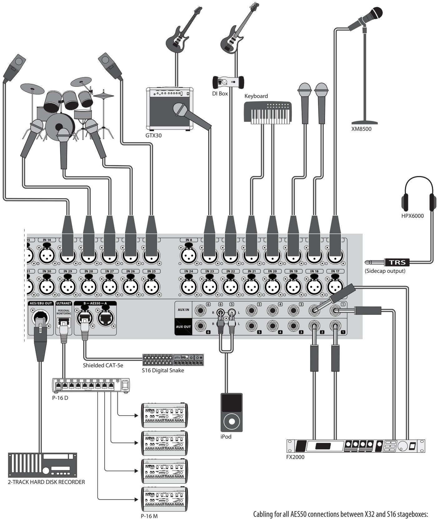
Cabling for all AES50 connections between X32 and S16 stageboxes:
