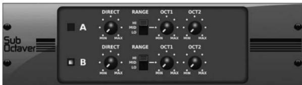
The Sub Octaver provides two channels of sub harmonics generation, one or even two octaves below the input signal.
