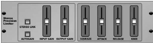
Stereo Precision Limiter allows you to set a precise volume limit, ensuring distortion-free, optimal signal integrity. Use X32's Stereo Precision Limiter to boost quiet signals or preventing clipping while preserving the level of "hot" signals.
