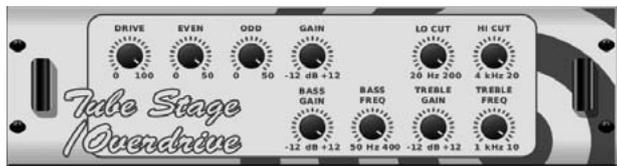
Tube Stage/Overdrive is a versatile effect capable of emulating a variety of modern and classic tube preamps. Available in stereo and dual-mono versions, use Tube Stage/Overdrive to dial in warm and fuzzy sounds from subtle to fully saturated.
