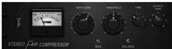
This model of a Fairchild 670 delivers some of the finest colorations in compressor history. Two small trim VRs, BIAS and BALANCE, preset the control side chain action, a 6-step knob determines the timing, and the 2 large INPUT GAIN and THRESHOLD knobs adjust the levels. There are models available for dual, stereo-linked, or mid/side operation.
