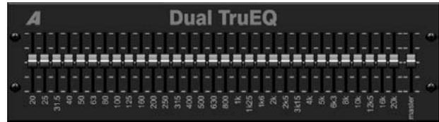
The TruEQ incorporates a special algorithm that compensates for the gain adjustment overlapping effect that adjacent frequency bands have on one another. On a standard EQ, when neighboring bands are boosted together, the resulting effect is magnified beyond what is visible from the positioning of the sliders.
