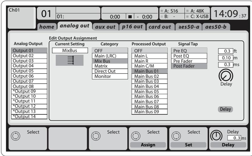
**Output Signals** can be freely assigned from any internal signal to any of the following outputs:
