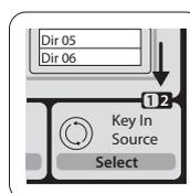
Some of the individual pages on the main display contain more adjustable parameters than can be controlled by the 6 rotary push encoders located beneath it. In these cases there is a small page number indication, e.g. "1/2". Simply press the Layer Up/Down buttons to switch between layers.
