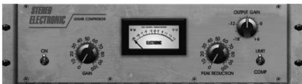
This model of a popular tube-based optical compressor provides natural and effortlessly musical compression, inspired by the Teletronix LA-2A. Simply adjust the input GAIN and PEAK REDUCTION knob to dial in the amount of desired compression, then adjust the OUTPUT GAIN knob for the desired output level. The COMP setting will give a gentle compression ratio, whereas the LIMIT setting results in a higher ratio.
