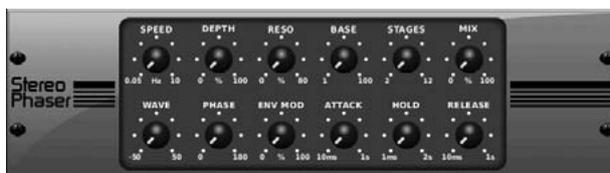
A Stereo Phaser, or phase shifter, applies multiple STAGES of modulated filters to the input signal to create a "notch" in the frequency response, and then applies a MIX with the original for a "swirling" effect. Use X32's Stereo Phaser to add a "spaced-out" sound to vocal or instrument tracks.
