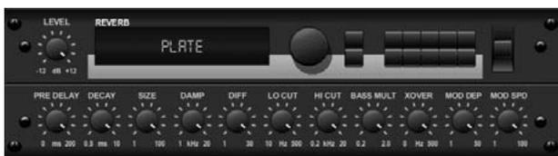
A plate reverb was originally created by sending a signal through a transducer to create vibrations on a plate of sheet metal which were then picked up as an audio signal. Our algorithm simulates that sound with high initial diffusion and a bright colored sound. X32's Plate Reverb will give your tracks the sound heard on countless hit records since the late 1950s. (Inspired by the Lexicon PCM-70)
