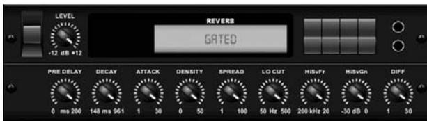
This effect was originally achieved by combining a reverb with a noise gate. Our gated reverb creates the same impression by a special shaping of the reverb tail.
