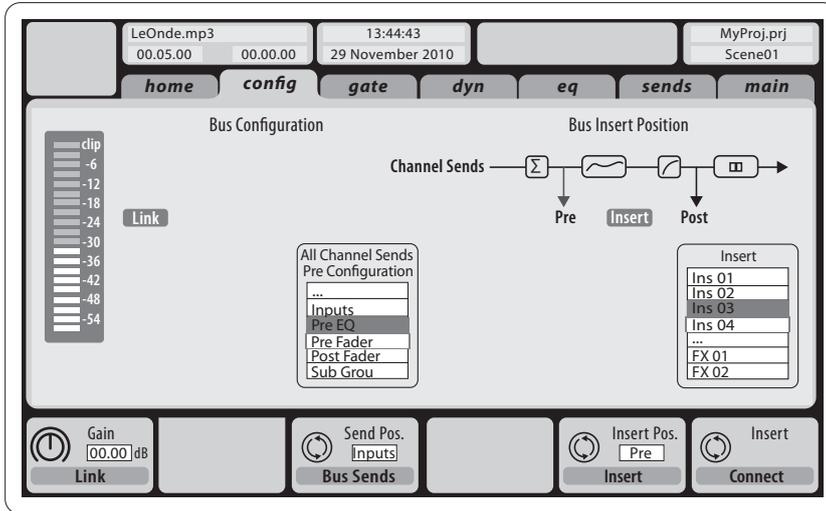
The configuration of **Mix Bus Channels 1-16** can be pre-set (in the Setup/Global page) or can also be configured on an individual, per-channel basis. The bus processing includes (in this order):
